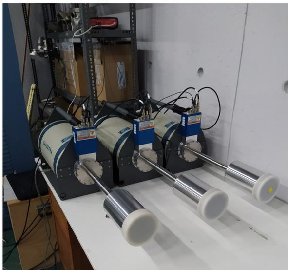
*Figure 2.1.1: The three CANBERRA HPGe detectors.*
