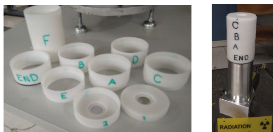
Picture 3.3: The spacers used to fix the source-detector distances (left) and some of them in use (right).
