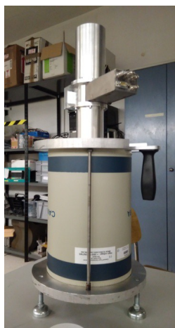
Picture 3.1: The CANBERRA EGPC 25S/N 54035 p-type coaxial HPGe detector mounted on its holder.
