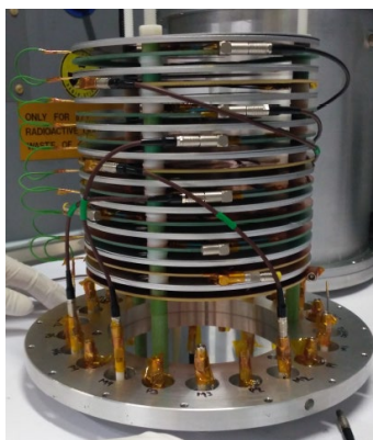
Figure 1.10: The stack of detectors and samples [18].
