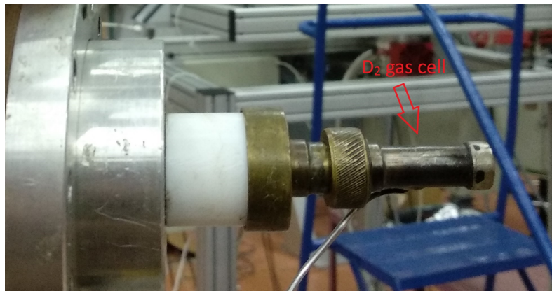
Figure 3.2: The lateral view of the D_2 gas cell at the accelerator facility of “Demokritos”.
